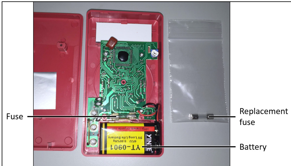
Figure 2. The back cover of the DMM removed to show the location of the battery and fuse.
